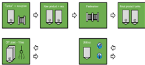
Block diagram unitised Pilot Process Plant
