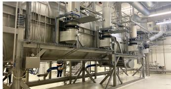
To ensure the correct heat treatment of the product, a critical control point (CCP) system was implemented on the evaporator.
